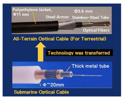
Figure 1 Example of L.110 cable (upper one) used for the solution BIR
