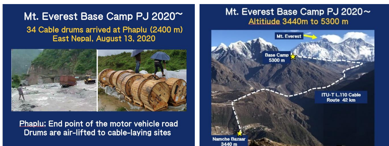
Figure 5. The cable drums arrived at the site, and the cable route
