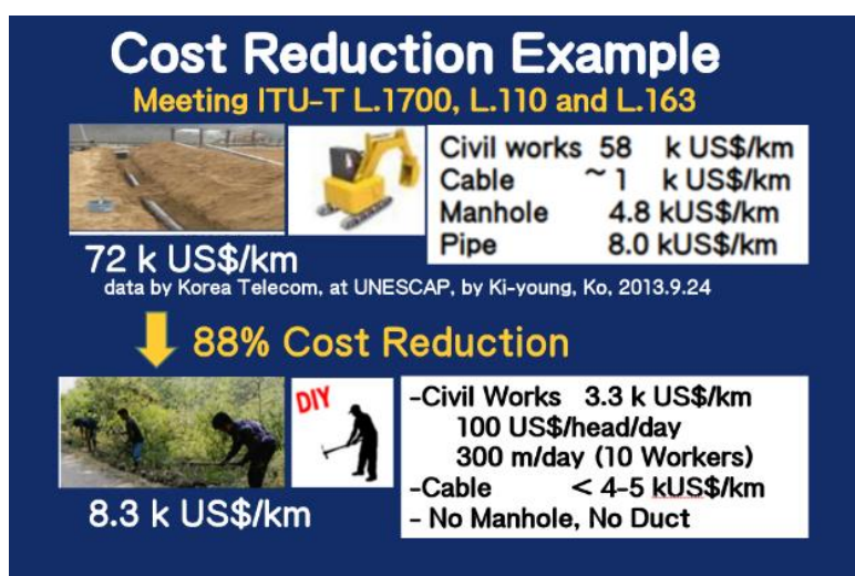
Figure 2. Cost Reduction example of L.110 Cable and its construction
